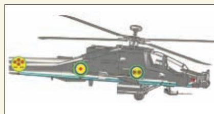
▲ Fig. 2 Model of a cable harness inside an Apache helicopter for EMP analysis: inset pictures show the cable cross-section at different locations.
